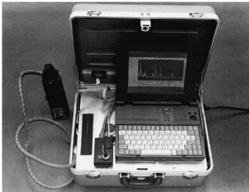
Fig. 3. Photographic detail of the first portable LIBS analyzer designed by Cremers et al. [28]. Published with the permission of the Society for Applied Spectroscopy.
